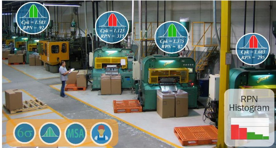
Figure 88 Conceptualization of using AR application for KPIs visualization on a full productive line [389].
