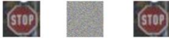
Figure 21. Stop sign before perturbation, perturbation and adversarial example (adding perturbation) classified as speed limit of 60 km/h by ResNet model [Source: Suo et al., 2019].
