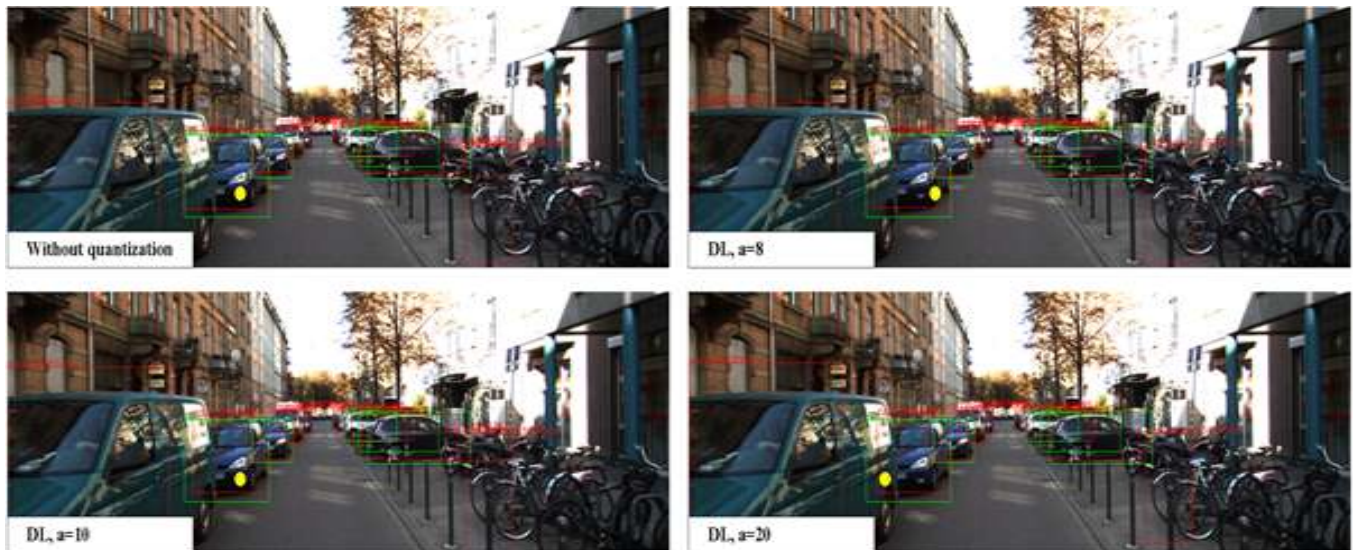
Figure 37: Application of accelerated vs original SqueezeDet models, using examples from the KITTI dataset. Green rectangles correspond to ground truth boxes, while red rectangles to predictions. The confidence scores are also shown in red letters. Yellow rectangles in (a) and yellow dot in (b) highlight the most obvious performance degradation of the accelerated networks, as compared to the original one.
