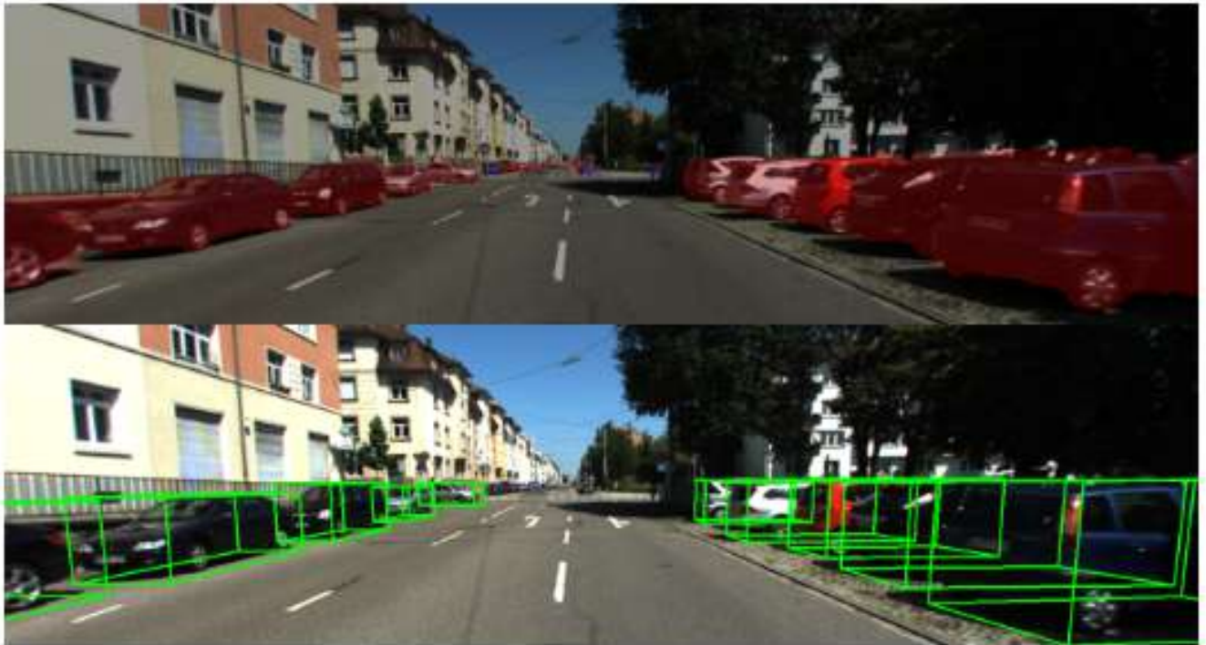
Figure 26: From top to bottom: 2D segmentation output and 3D detected objects projected to the image plane.
