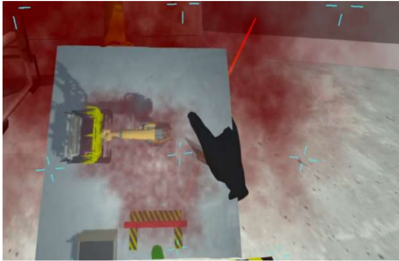
Figure 13: Example of safety zones and collision risk in space.
