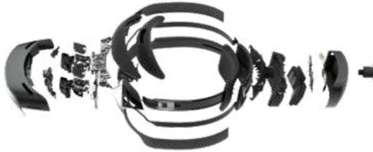
Figure 54: Microsoft HoloLens 2: components
