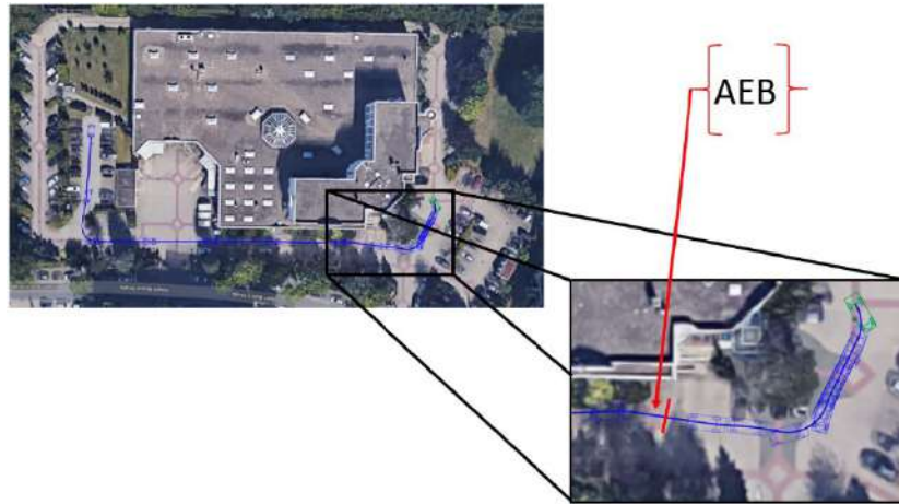
Figure 26: Avoiding a collision while following a path for a test vehicle
