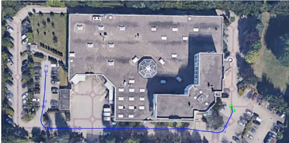
Figure 24: Planning a global path for a test vehicle in Panasonic Automotive building to go to the Parking area using Hybrid A*
