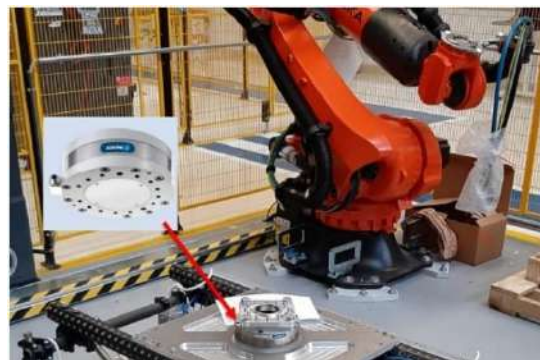
Figure 7: Force-Torque Sensor FTN – Omega 191 assembled on the gripper before final assembly
