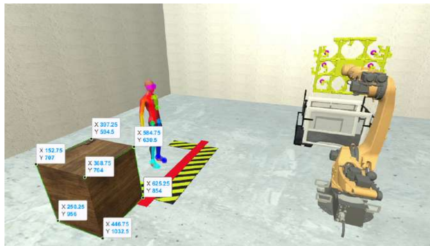
Figure 15: Recognition of box corners and estimation of their coordinates.
