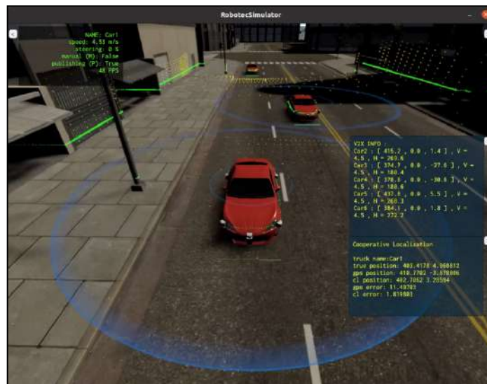
Figure 46: RoSi view of V2X messages together with GPS and Cooperative Localization errors.
