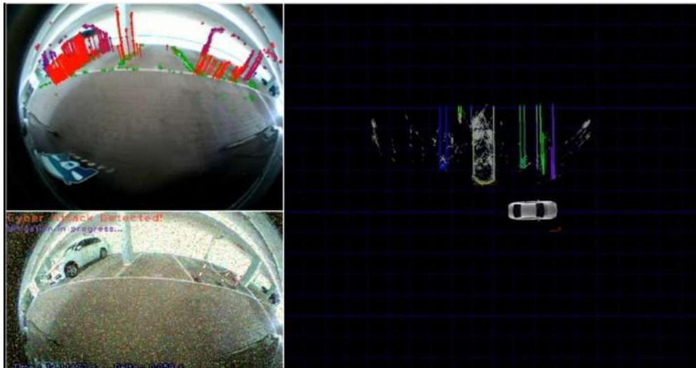
Figure 115: Output of boundary estimation while the camera is cyber attacked. Top left: Output of 3D environmental sensing. Bottom left: Cyber attack at the camera sensor. Right image: Polygons enclosing the point clouds clustered as discrete objects.
