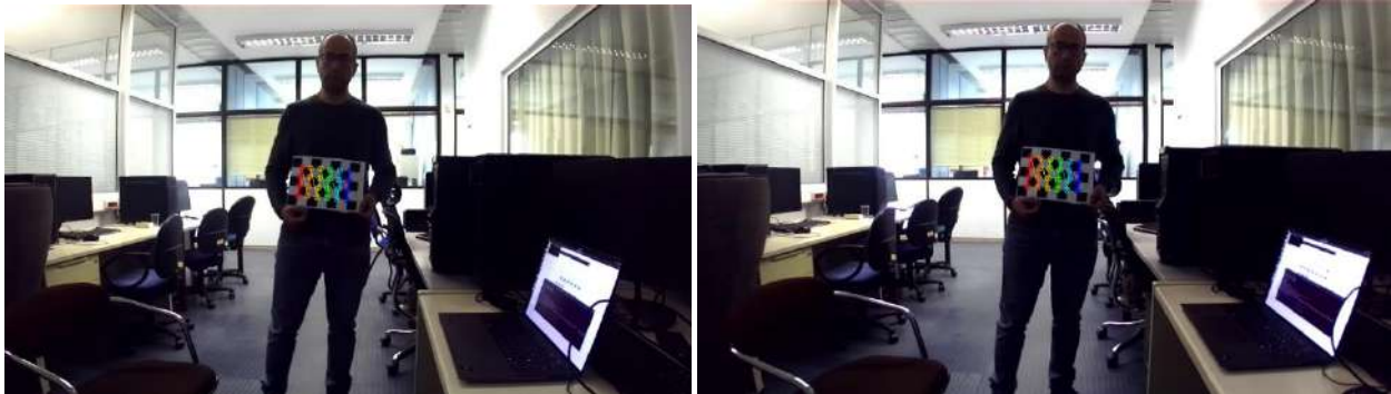
Figure 35: Example of the left and right camera calibration.
