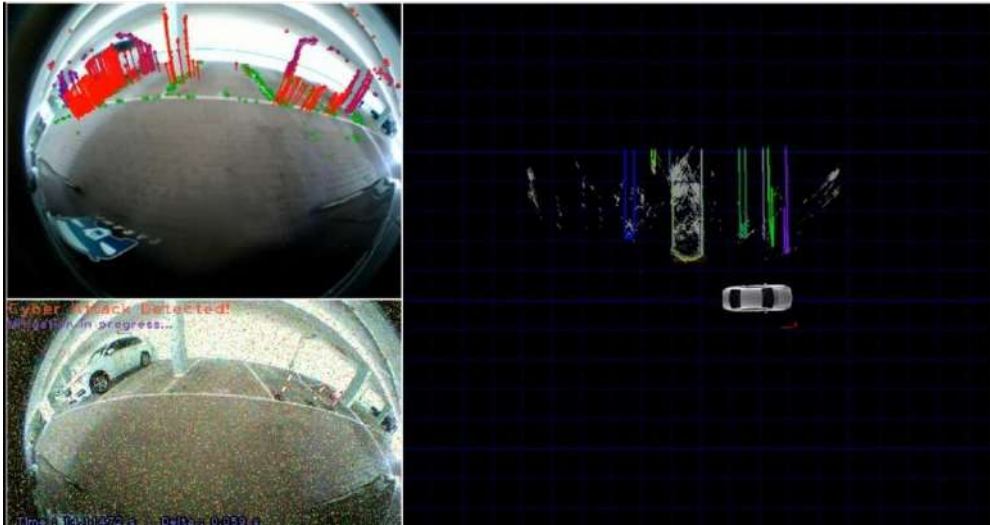
Figure 117: Output of boundary estimation while the camera is cyber attacked. Top left: Output of 3D environmental sensing. Bottom left: Cyber-attack at the camera sensor. Right image: Polygons enclosing the point clouds clustered as discrete objects.
